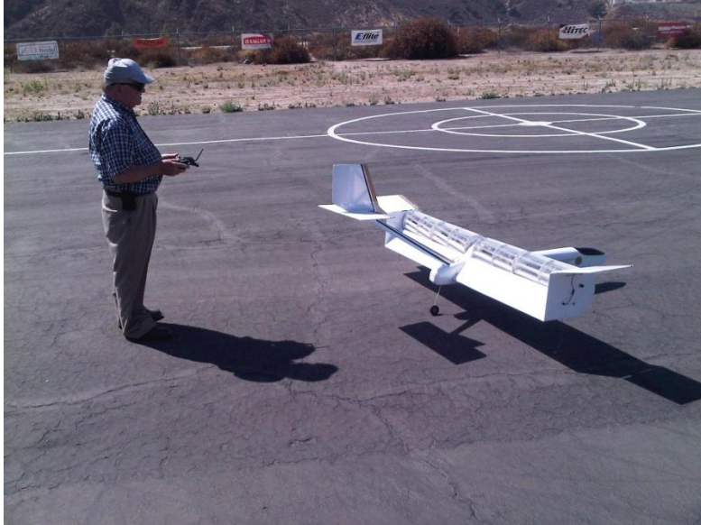
Jack Vail's Fanwing. 8 foot wingspan, hacker 70L, flies on 6S.
